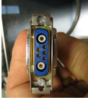
Figure 37 RF Generator cable connector.
