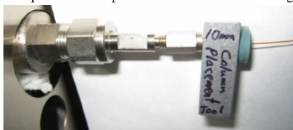
Figure 18 The 10 mm positioning tool (Gauge) in place.
