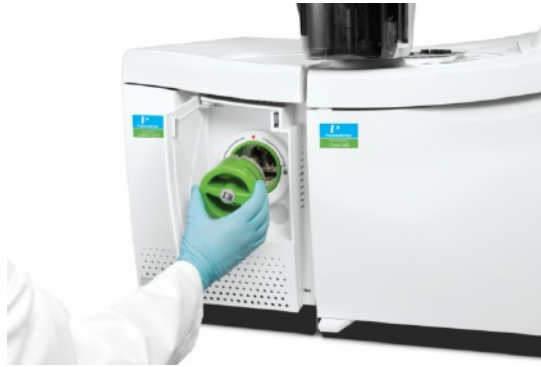
Figure 11 Removing the source.
