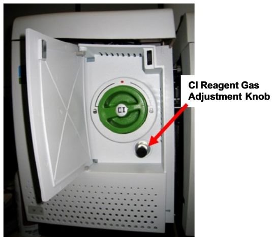
Figure 45 CI reagent gas adjustment knob.
