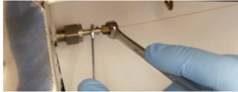
Figure 17 Tightening the column nut.
