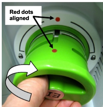
Figure 13 Lining up the red dots.
