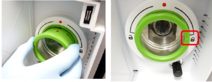
Figure 19 Inserting the Plug Handle and Sight.
